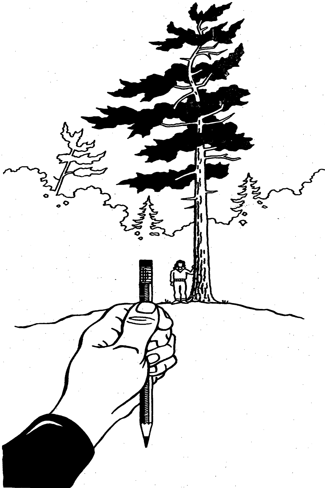
Figure 5: Estimating the height of a tree is made easy using the proportional method illustrated below.
